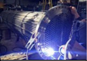
HEAT EXCHANGER MANUFACTURING
